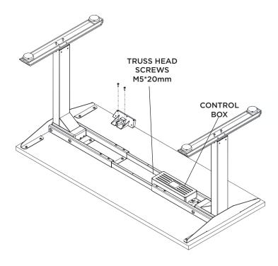
**Step 4:** Disconnect wiring and slide the control box out from its housing. Replace with new control box.
