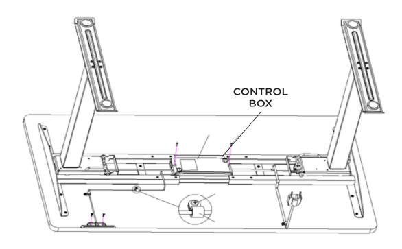
Step 2: Unwedge the control box from the frame. Replace with new control box
