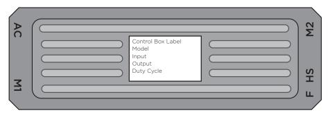
AC - Power Cord M1, M2 - Leg cables HS - Display Cable F - N/A
