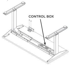
NOTE: The control box must be installed with the label facing outwards.
