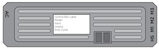
AC - Power Cord M1, M2, M3 - Leg cables HS - Display Cable
