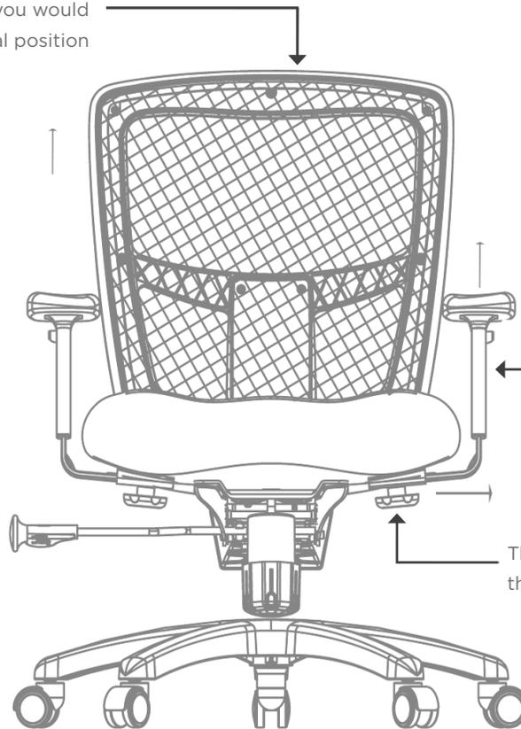
Press this button to adjust the up and down of the armrest
