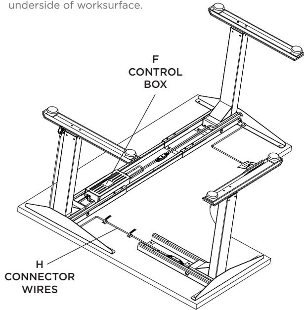
Schematic view of the My-Hite wiring:
