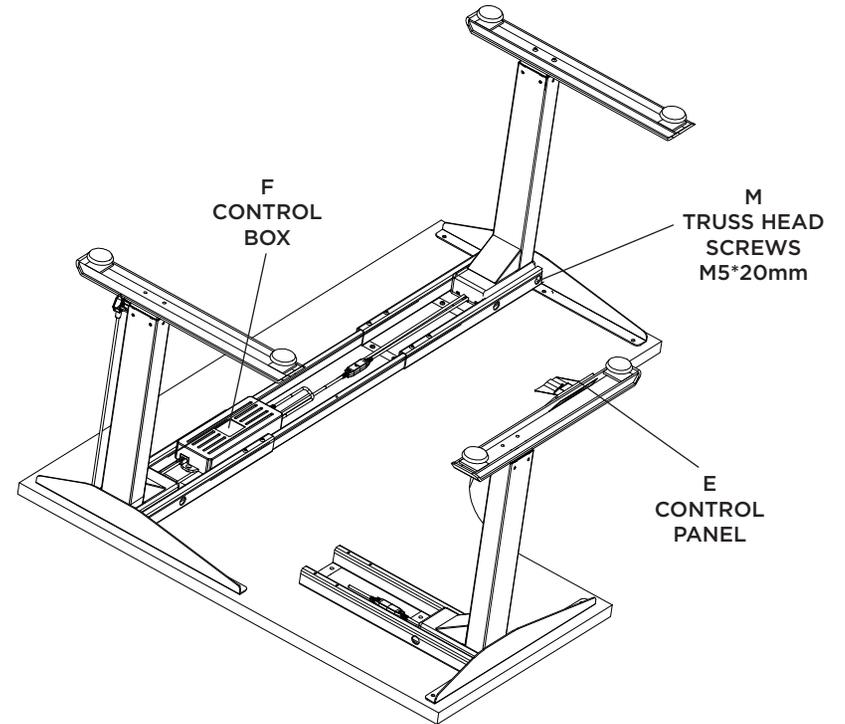
**Step 11:** Insert the **F** control box in-between crossbeams.
