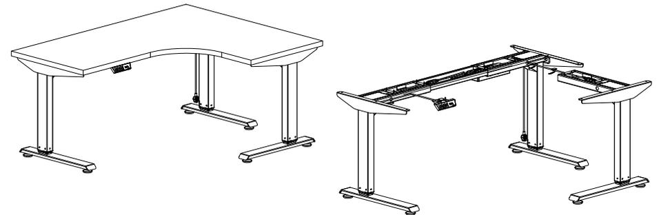
**Step 14:** Turn table right side up, adjust the glides as necessary, and plug the power cord into a 110v outlet.
