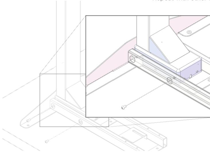
**Step 5:** Remove **D** pad after leg installation, then reuse for assembly of other leg(s) repeating steps 3 & 4. **Remove pad when done.**
