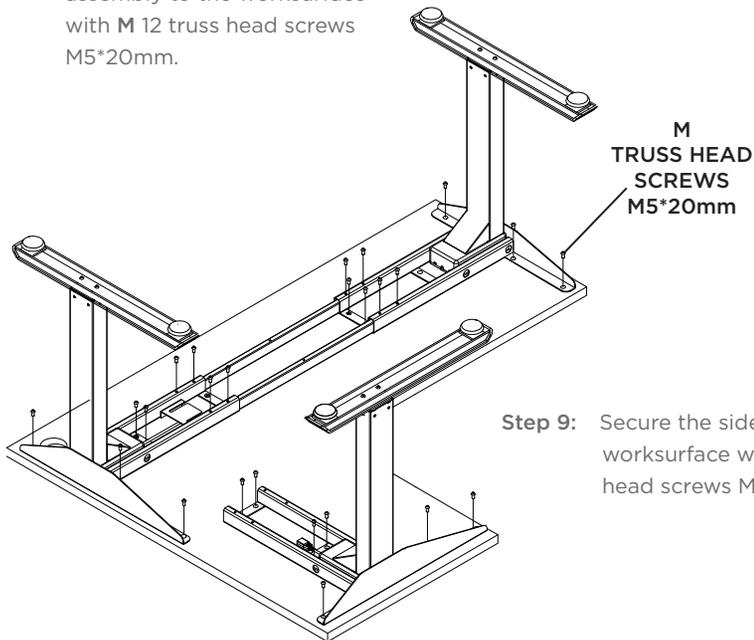
**Step 9:** Secure the side bracket to the worksurface with **M** 12 truss head screws M5\*20mm.
